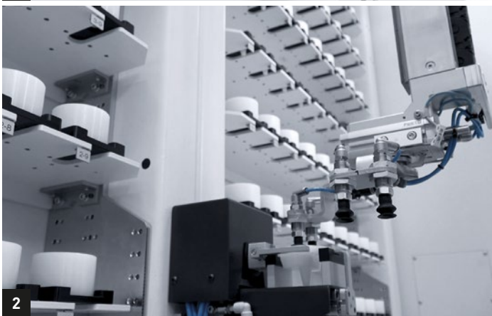
1.+2. PH 10 version as a workpiece handling system for up to 126 raw parts and finished tibia components.
