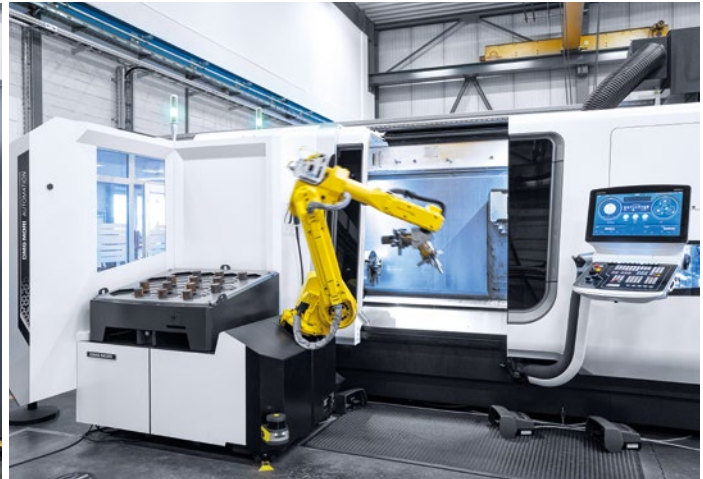
Automated 6-sided complete machining on the CTX beta 1250 TC reduces the machining time for the workpieces to 1.5 hours, a reduction of up to 80%.
