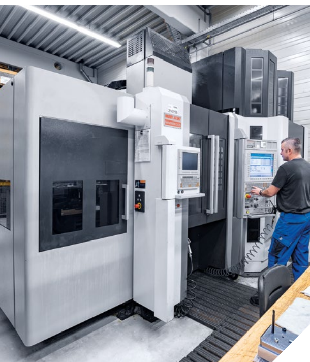
Loll Feinmechanik uses three 5-axis NMV 3000 machining centers each equipped with a 34-station AWC 34 pallet handling system for the flexible production of one-offs and small batches.
