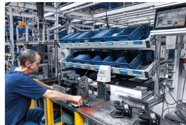
A test station determines torques during assembly and the data is recorded in the TULIP APP for subsequent analysis.
