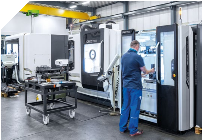
The PH 150 on the CMX 70 U enables automated machining of small batches and one-offs with needs-based prioritization.
