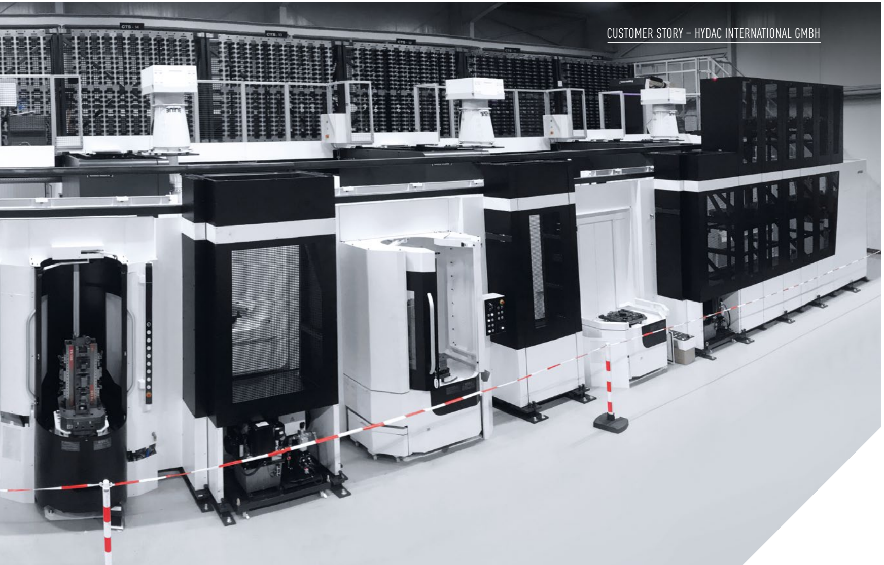
The six NHX 4000s with storage for 48 pallets form an automated system more than 33 m wide. A tool magazine with up to 4,000 pockets has also been integrated into the system.
