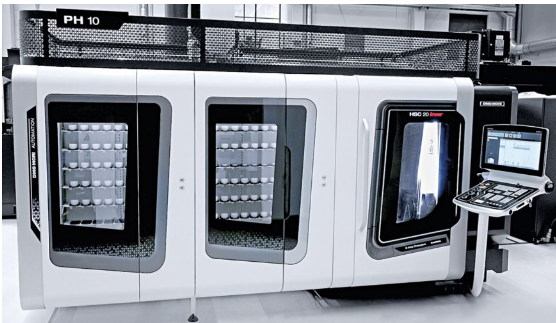
HSC 20 linear with a dual version of the PH 10 as a workpiece handling system
